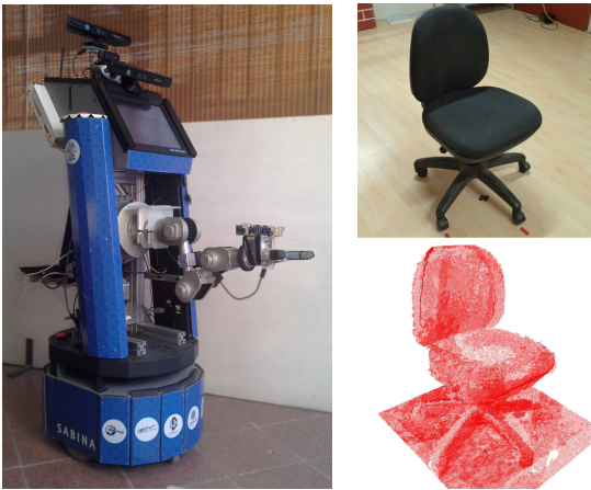
Fig. 1 The proposed method is able to plan each robot view/state in order to reconstruct a real object. In our experiments we use a mobile manipulator of 8 degrees of freedom to reconstruct several objects. A Kinect sensor was mounted on the robot’s end effector.
