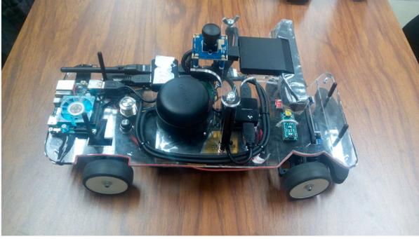
Figure 17. The car-like robot and the sensors.
