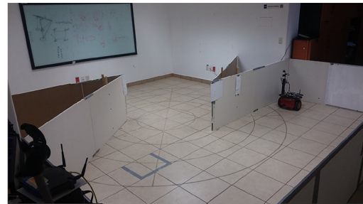
(a) Lab: This environment is a drywall made structure in the CIMAT robotics lab, it is composed of 6 straight line segments, 8 concave corners and 2 convex corners
