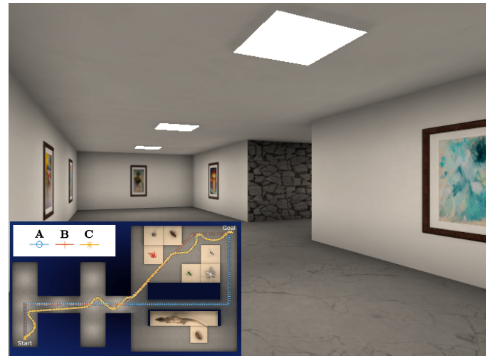
Fig. 4. A screenshot from the museum environment used in the user study. A top-down view of the museum is also shown along with three tested trajectories. Pareto trajectory that minimizes the number of rotations is labeled as A. Pareto trajectory that focus on reducing distance is labeled as B. The tested RRT trajectory is labeled as C.
