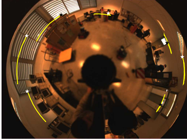
Fig. 12. Some of the tracked points (stars) and their motion in the image along a sequence.
