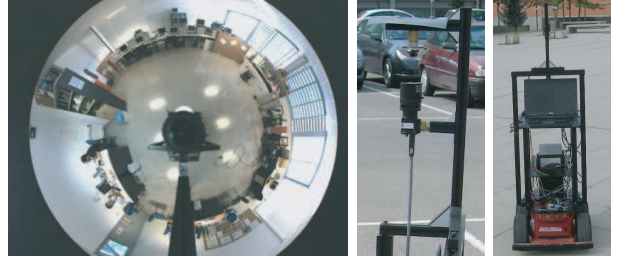
Fig. 10. Example image (left), omnidirectional camera (center) and complete setup (right) used for the experiments.
