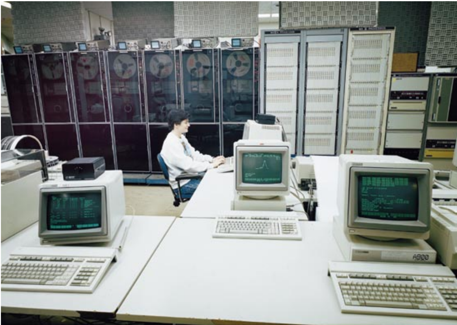
The Mark III and Mark IIIA processors at Haystack are shown together with playback recorders and computer control and monitoring terminals.
