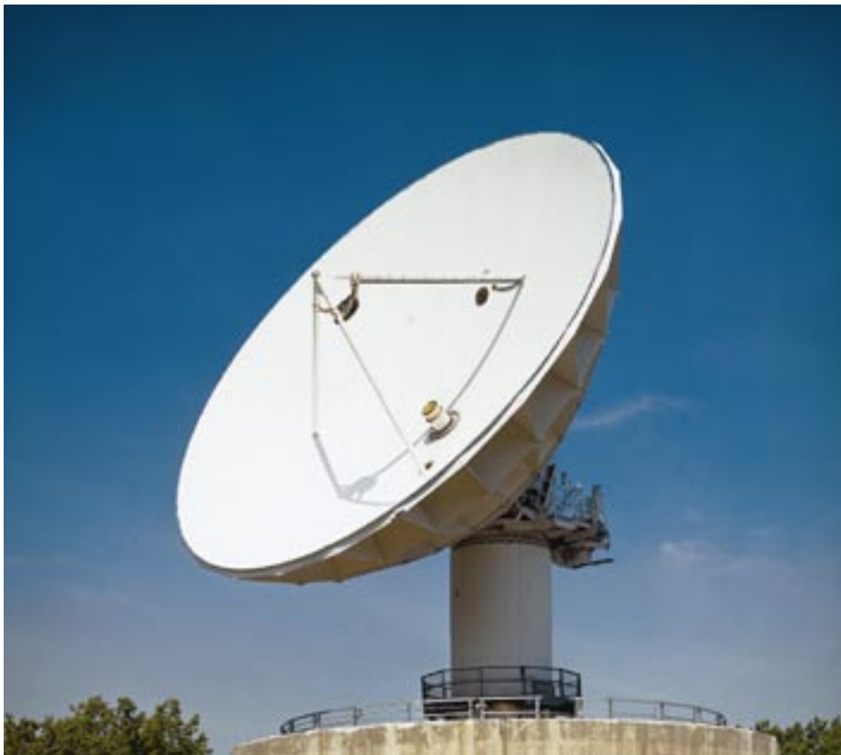
The Westford radio telescope is an 18-m diameter antenna enclosed in an inflatable radome (not shown here) and operates with radiometers at frequencies of 2.8 and 8.4 GHz as part of the VLBI geodetic network.
