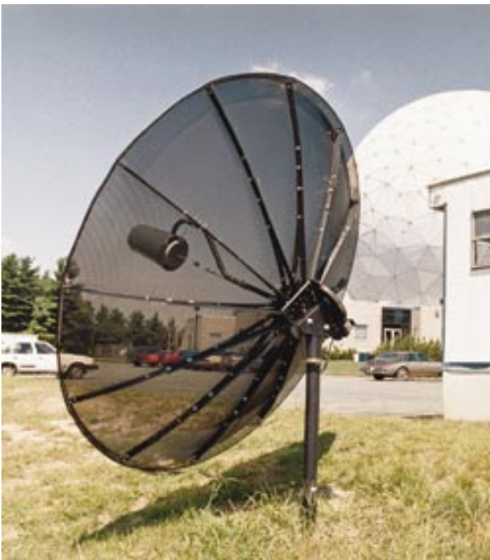
A 3-m diameter small radio telescope using a TV satellite dish has been developed at Haystack as an educational tool for radio astronomy.
