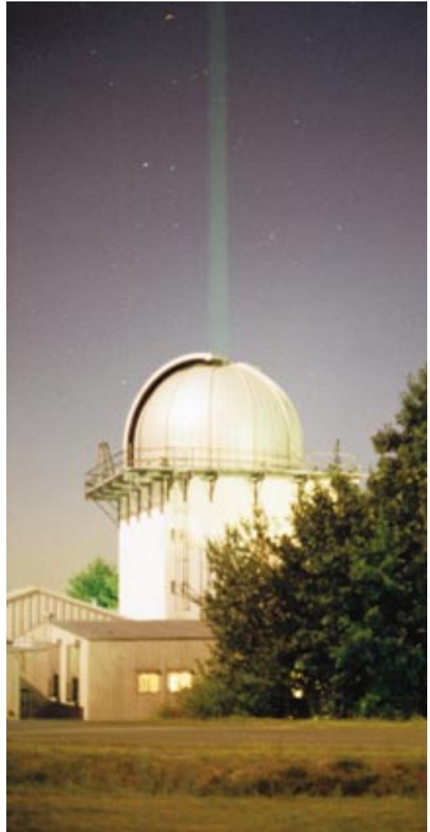
The laser beam of 800 milli-Joule intensity emitted from the Firepond 1.2-m optical telescope in experiments to demonstrate the capability of the system to study the structure of the stratosphere and mesosphere.
